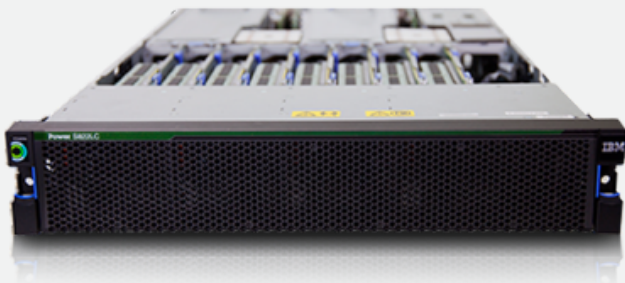
Figure 1. IBM Power NVLINK server with 4 NVIDIA Tesla P100 GPUs used for running ECHELON.
