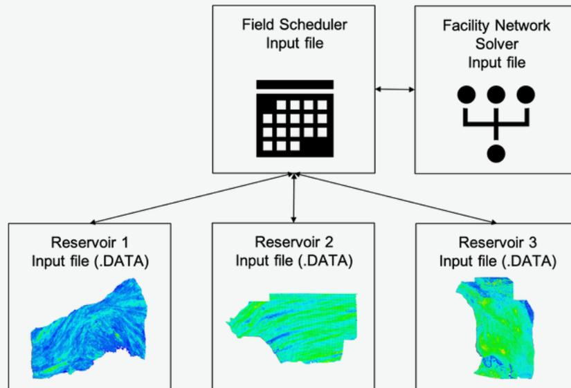
Standalone ECHELON simulation models can easily be coupled through the field scheduler to balance groups producing from multiple reservoirs. No change to the static and well properties parts of the .DATA files is required. The field scheduler seamlessly connects to the integrated facility network solver, to self-consistently model the impact of network backpressure on the wells.
